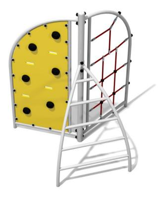
Climbing equipment consisting of two walls and curved ladder. First wall is filled with 19 mm HDPE plate with climbing stones. Second climbing wall consists of reinforced 16mm rope. The structure is hot-dip galvanized and powder painted.
